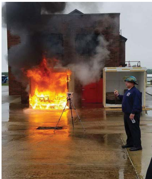
A moderately furnished room without sprinklers at the 3-minute mark. The room is beyond survivability and would be threatening the entire home at this stage.
